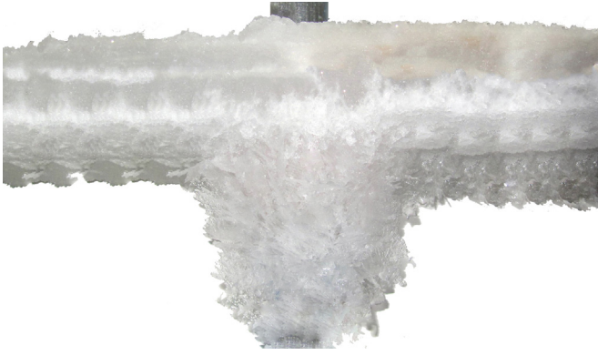
Fig. 1. Ice collar on the vertical cylindrical pipe submerged in the marine water.
