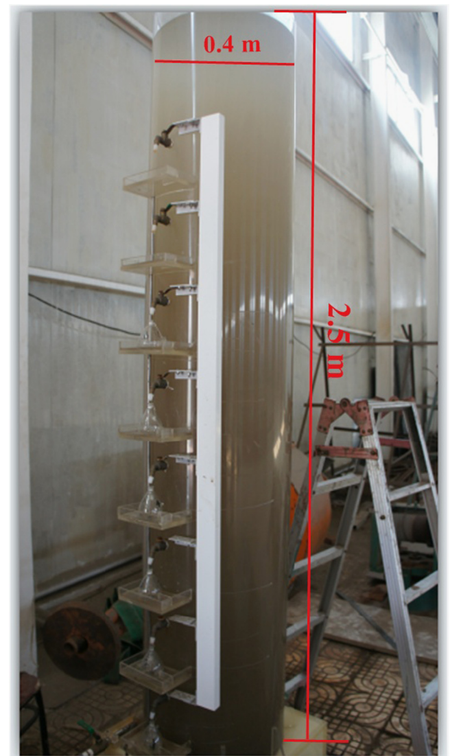
Fig. 1. Photo of a traditional settling column, the outlets are connected together to a shaft to insure simultaneous sampling (Photo courtesy: HUANG Wei).
