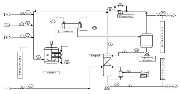
Fig. 1. The Tennessee-Eastman process (TEP).
