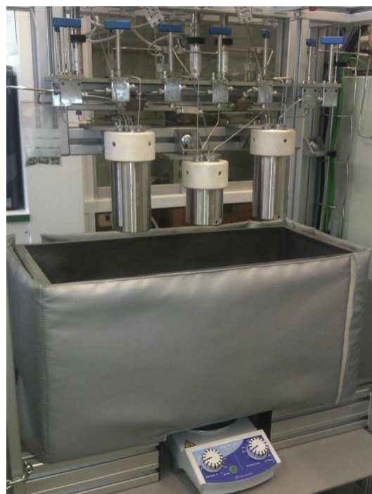
Fig. 2. Two 191 cm 3 and one 111 cm 3 pressure vessels of the gas dosing system and their connections above a temperature controlled bath.
