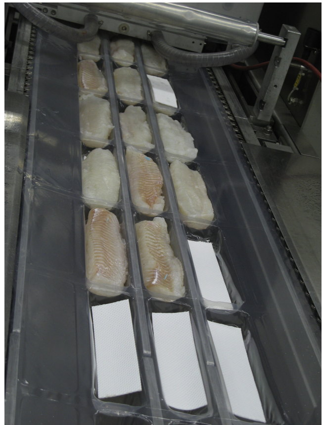
Fig. 1. Packaging of cod loins in a thermoforming machine for modified atmosphere packaging (MAP) and vacuum packaging, using either liquid absorbing pad (picture) or a CO 2 emitter pad.
