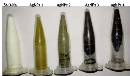
Fig. 1. Photographic photo of the powdered AgNPs prepared at different concentrations of \text{AgNO}_3 , viz, (0 mM, 0.1 mM, 0.5 mM, 1 mM and 2) for St-ONa, AgNPs 1, AgNPs 2, AgNPs 3 and AgNPs 4 respectively.
