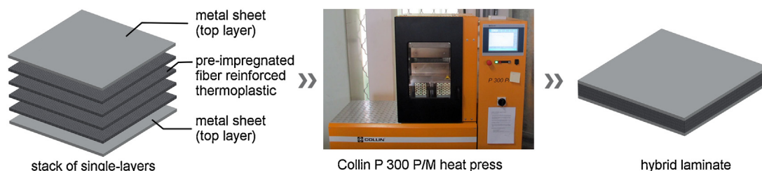
Fig. 1 – Structure of continuous fiber reinforced metal/composite-laminates.
