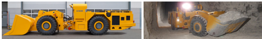
Fig. 1 – Self-propelled underground loader with the operator's cab.
