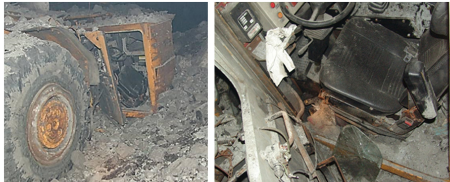
Fig. 2 – The operator's cab from outside (left) and inside (right) after the accident in KGHM Rudna.
