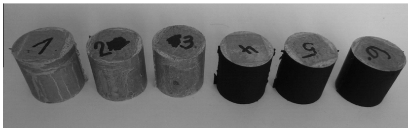
Fig. 1. Cylindrical specimens of integral-skin aluminium alloy foams.
