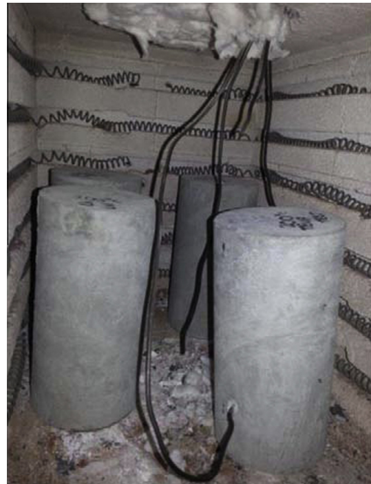
Fig. 1. Positions of type K thermocouples inside the kiln and in the cylinder.
