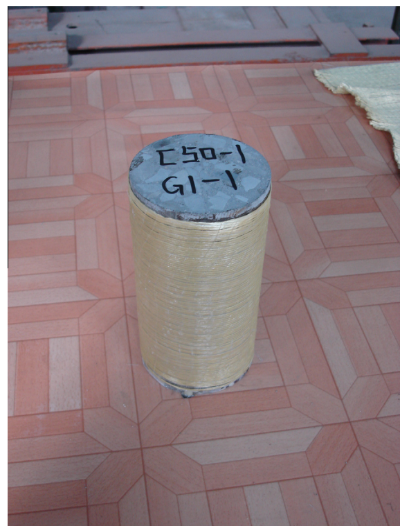
Fig. 2a. Typical specimen for quasi-static test.
