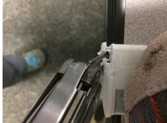
Figure 3. Remove the bottom of the casing.
