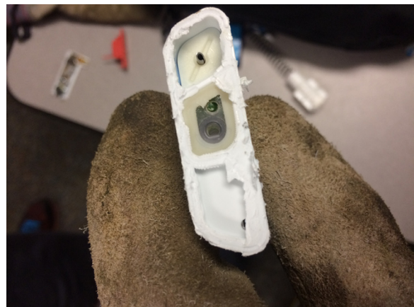
Figure 4. Remove the rubber seal.
