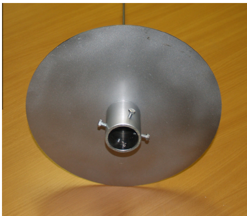
Fig. 2. The view of masts mounting to the aerodynamic balance.
