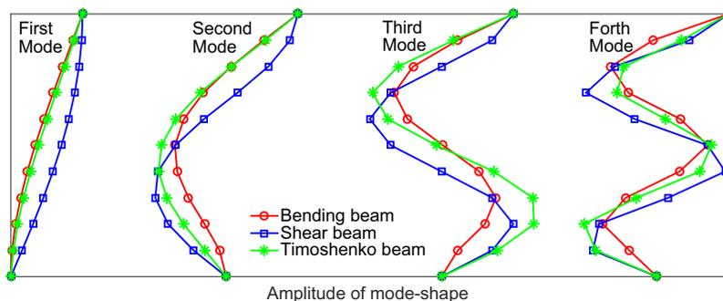
Fig. 1. The first four normalized mode shapes of the inverted bending, shear, and Timoshenko beams. Due to the differences in boundary conditions, all the beam models result in different mode shapes: curvature, amplitude, local maximum along the length of the beam, and the shape of the modes.
