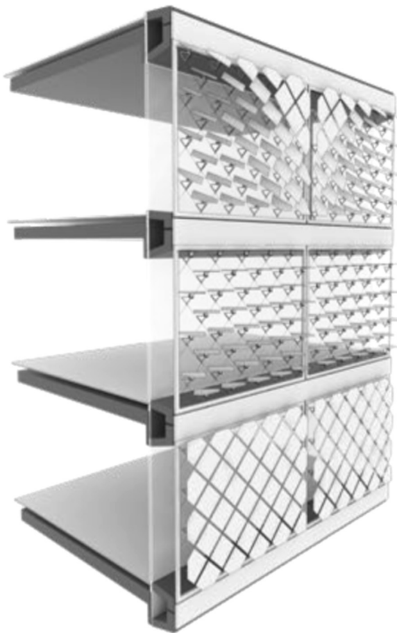
Fig. 2 Modules on a building facade, mounted in frames on a cable net structure within the shading layer of the facade.
