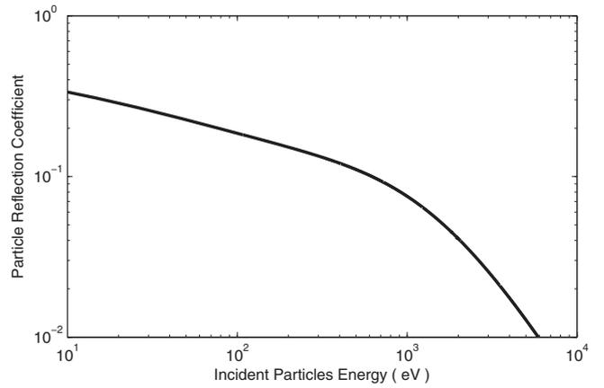
Fig. 2. Particles reflection coefficient versus incident particles energy on carbon wall.
