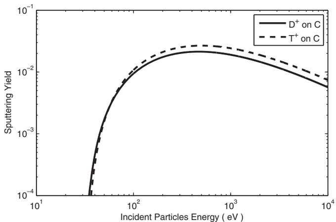
Fig. 1. Sputtering yield for deuterium and tritium ions incident on carbon wall surface.
