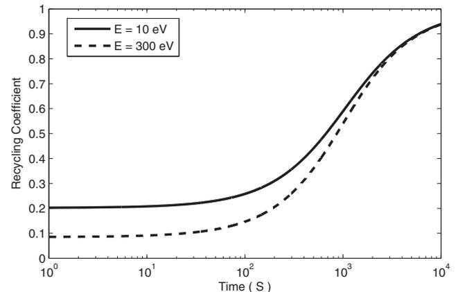
Fig. 3. Recycling coefficient over time in 10–300 eV incident particles energy.
