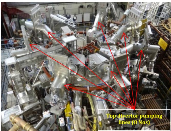
Fig. 1. Snap-shot of SST-1 tokamak with divertor pumping lines.
