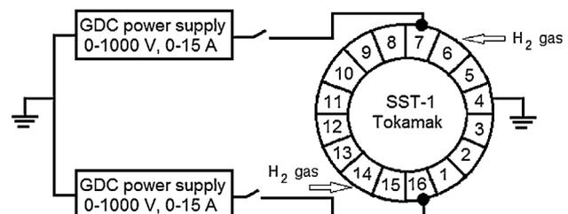
Fig. 2. GDC system installed at radial ports (R-7 & R-16) of SST-1.
