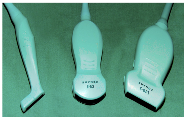
Figure 3 A selection of ultrasound scanning probes commonly used in regional anaesthesia. From (L) to (R) high-frequency linear probe with small footprint, low- to mid-frequency curve-linear and high-frequency linear probes.
