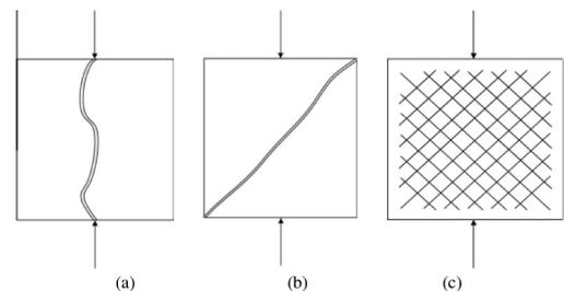
**Fig. 2.** Failure characteristics of concrete under uniaxial compression.
