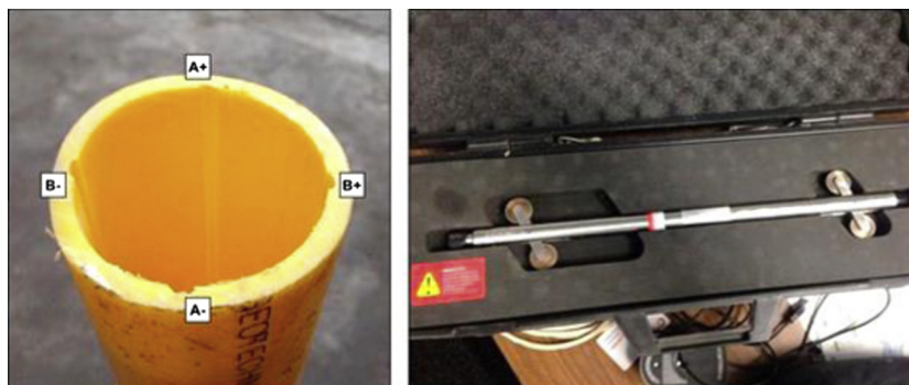
Fig. 2. Photograph of inclinometer casing and inclinometer probe.
