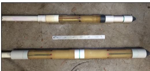
Fig. 2. Instrument assembly for the double 58 mm ANZI stress cell and the single 48 mm ANZI stress cell.
