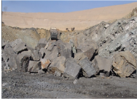
Fig. 2. Over-sized rocks (boulders) in a typical Golegohar's blast operation.
