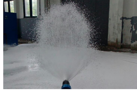
Fig. 2. Jet shape of arc jet nozzle.
