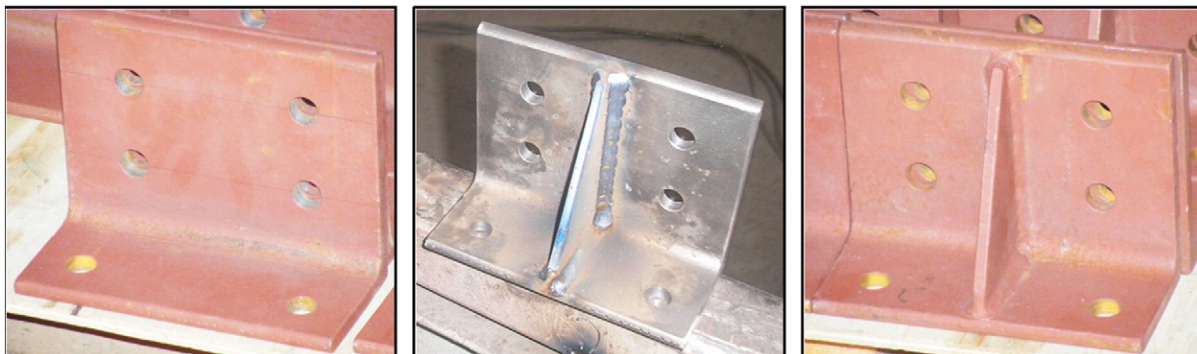
Fig. 2. Unstiffened and stiffened cleats.
