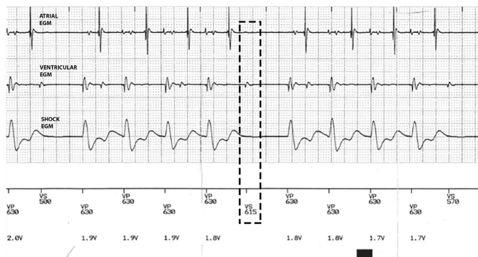
Fig. 2 – EGM post DFT threshold testing showing ventricular over-sensing of the artefact during pacing threshold testing (denoted by rectangular box showing that the artefacts are now being sensed by the device as VS, on the marker channel). EGM channels for both upper and lower panels: First line = Atrial EGM, Second line = Ventricular EGM, Third line = Shock EGM (distal coil to can), Fourth line = Atrial and ventricular pace/sense marker channel. Fifth line = Pacing output. AS = Atrial Sensed Beat, VS = Ventricular Sensed Beat, VP = Ventricular Paced Beat.
