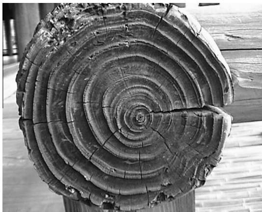
Fig. 1. The photodegraded cross section of an old temple fence part. (Myajima island, Japan).
