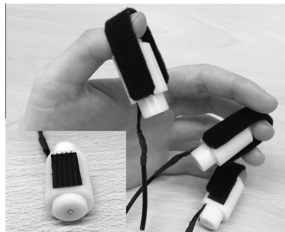
Fig. 1. Tactile stimulators attached to the thumb, middle finger and little finger of the left hand. The inset shows an enlarged view of one stimulator with the pin protruding from the stimulator.
