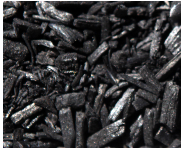
Fig. 1. Pieces of coarse miscanthus biochar, as ploughed into the field. The particle size ranges from a few millimetres to one centimetre.
