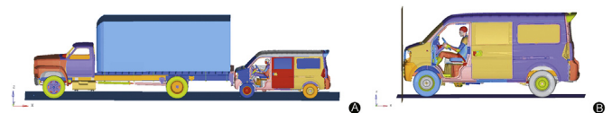
Fig. 2. Two collision models. A: The rear-end collision between the minibus and the truck. B: The head-on collision of the minibus to the rigid wall.
