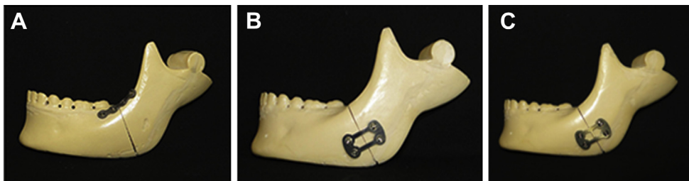
Fig. 1. A: The Champy fixation technique representing group I. B: The 4-hole grid plate representing group II. C: The 4-hole grid plate with the middle reinforcement vertical bar representing group III.
