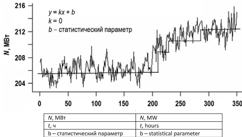
Fig. 1. Existing approach to forecasting energy consumption for coverage of plant needs at the SNPP.
