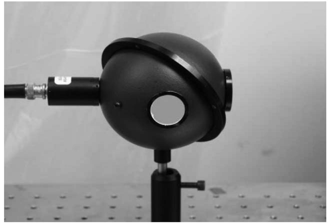
FIG. 1. Integrating sphere measures light transmission
