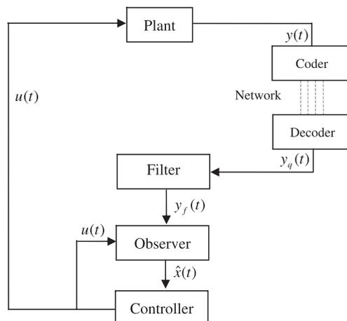
Fig. 1. The structure of a quantized system.
