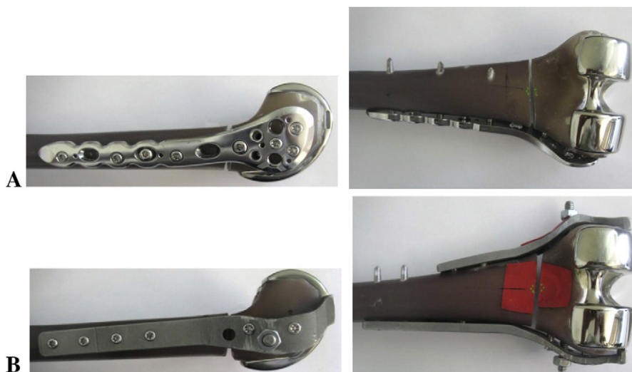
Fig. 1. Femur samples fixed with one of two options: (A) distal lateral femoral locking plate or (B) novel bilateral locking plates. The bilateral plates included a transverse compression screw through the femoral condyles and eight locking screws (four on the proximal lateral side, two on the distal lateral condyle, and two on the medial diaphysis). Tabs at the distal ends of the bilateral plates inserted into the existing slots on the sides of the femoral prosthesis.
