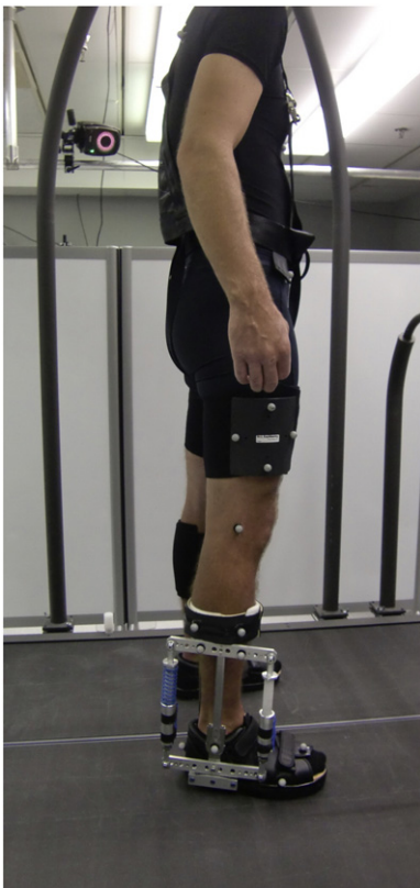
Fig. 1. Experimental setup using the custom experimental AFO, Bertec split-belt fully instrumented treadmill and Vicon 3-D motion analysis system.
