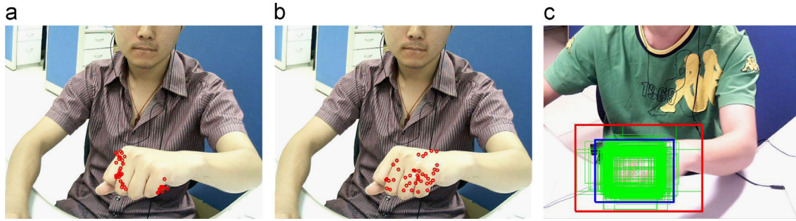
Fig. 1. (a) The feature points derived using Shi and Tomasi's algorithm. (b) The feature points derived using our method. (c) The small green bounding boxes are the particles generated in the current frame. The red bounding box is the smallest bounding box that contains all the particles. The blue rectangle is the tracking result. (For interpretation of the references to color in this figure caption, the reader is referred to the web version of this paper.)
