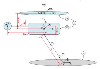
**Fig. 1.** Tethered helicopter scheme: description of reference frames, centers of mass and dimensions of interest for modeling purposes.
