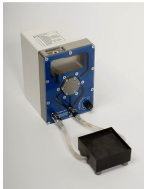
FIGURE 1. Flow simulator and single-vessel tissue phantom, Axiom Medical Ltd.
