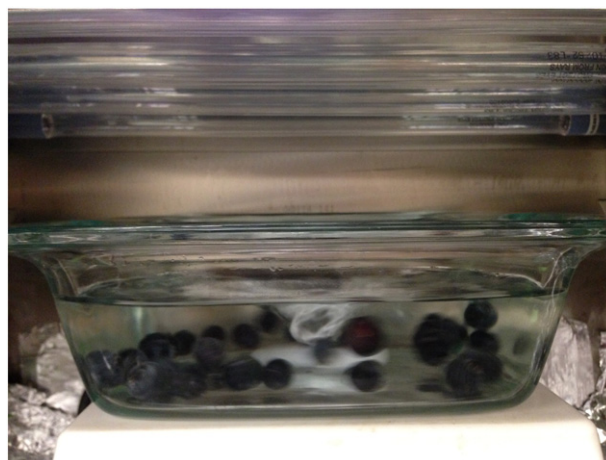
Fig. 1. Large-scale water-assisted UV treatment setup. UV lamps are on top of the chamber.
