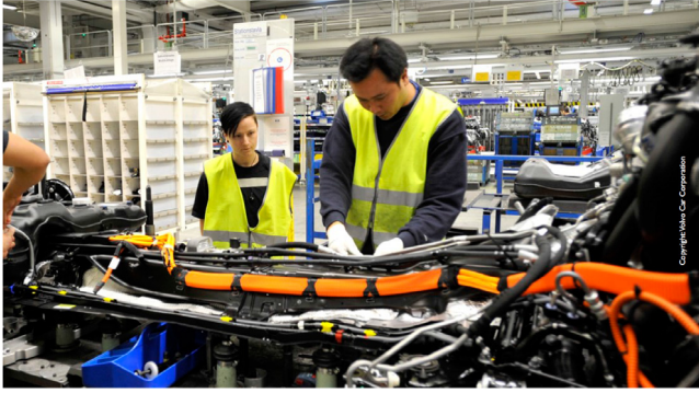
Fig. 1. Assembly of a high-voltage power cable in a hybrid car. © 2014, Volvo Car Corporation.
