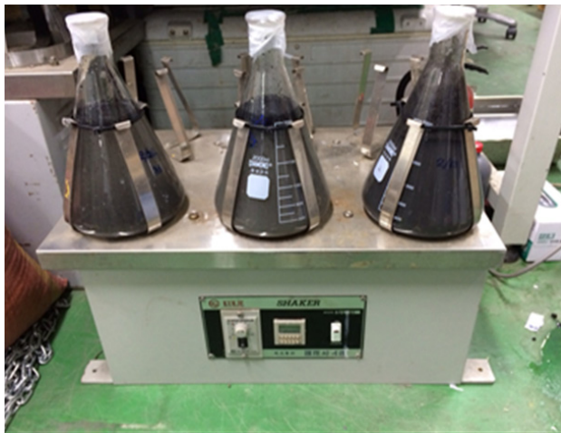
Fig. 1. Heavy metal leaching test
