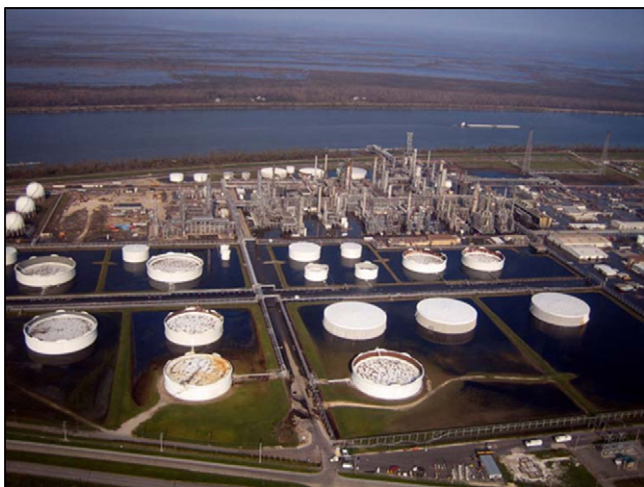
Fig. 1. Helicopter view (VIS camera) of breached oil containers near New Orleans (USA) after the hurricane Katrina episode, in August 2005. Note that is ambiguous the interpretation about the nature of the dark material around the tanks, which may be either water, oil or a mixture of both (source: U.S. Environmental Protection Agency— http://archive.epa.gov/katrina/web/html/photogallery.html ).
