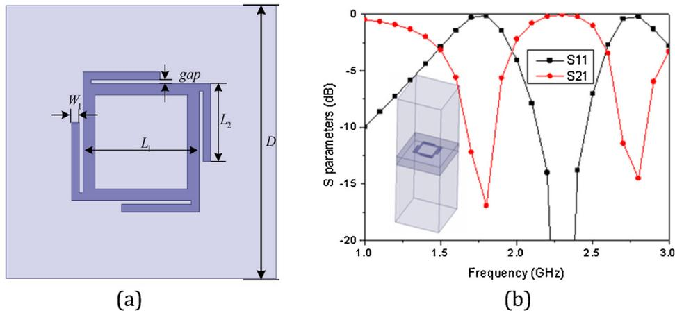
Fig. 1. Cell element of FSS (a) structure, (b) S parameters.
