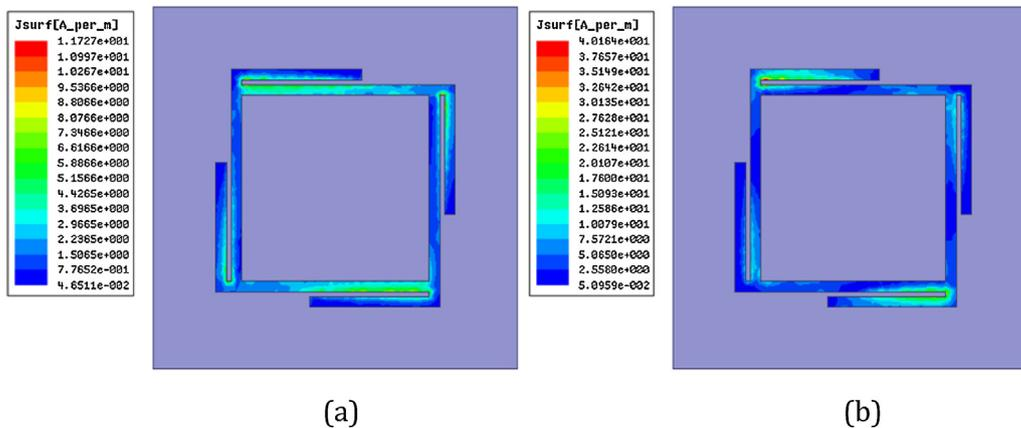
Fig. 2. Current distributions at different resonant frequencies. (a) 1.7 GHz and (b) 2.7 GHz.
