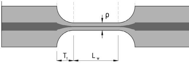
Fig. 1. Biconical tapered fiber.
