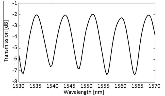
Fig. 2. Experimental transmission response of a biconical tapered fiber.
