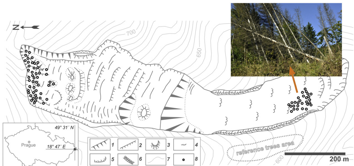
Fig. 1. Location and geomorphic map of the study area, and the view on the disturbed trees (1 – main scarp, 2 – minor scarp, 3 – partial landslide block, 4 – deformed surface of frontal lobe, 5 – border of frontal lobe, 6 – lateral levee, 7 – izoline (5 m), 8 – sampled tree).
