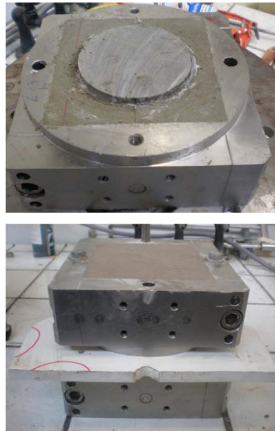
Fig. 2. Specimen preparation: marl specimen sealed with a mortar in one half box (top picture); the two half box assemblies ready to be installed in the shear box (bottom picture); dimensions of the boxes are 140 mm × 140 mm.
