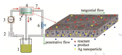
During cross-flow catalysis, products in penetrative flow are timely separated from the reactants in the tangential flow by the composite membrane.(1 feed tank; 2 diaphragm pump; 3 pressure guage; 4 membrane cell; 5 membrane; 6 valve; 7 tangential flow; 8 penetrative flow)
