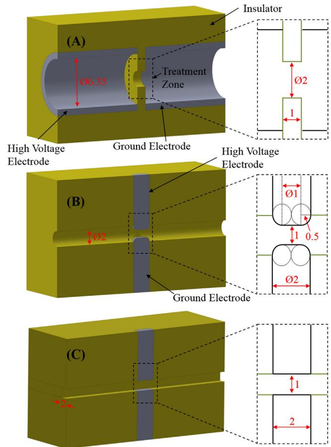
**Fig. 1.** Isometric views of treatment chambers sectioned through a longitudinal plane passing through the middle of the treatment zone. Liquid flows from left to right. Treatment chamber designs are: (A) Co-linear; (B) Steinmetz and (C) Parallel-plate. Dimensions are displayed in mm.
