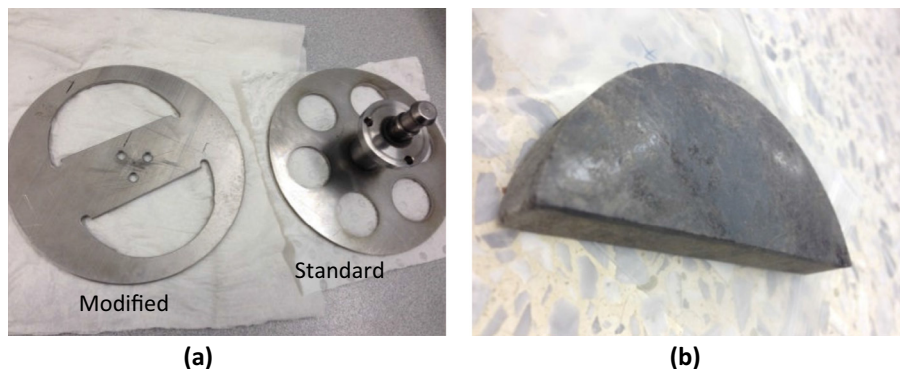
Fig. 3. (a) Specifically designed polishing foot to accommodate the slabs to be polished in the standard polisher and (b) a final polished slab 1 cm in thickness, 63.5 mm in diameter (Wightman et al., 2014).
