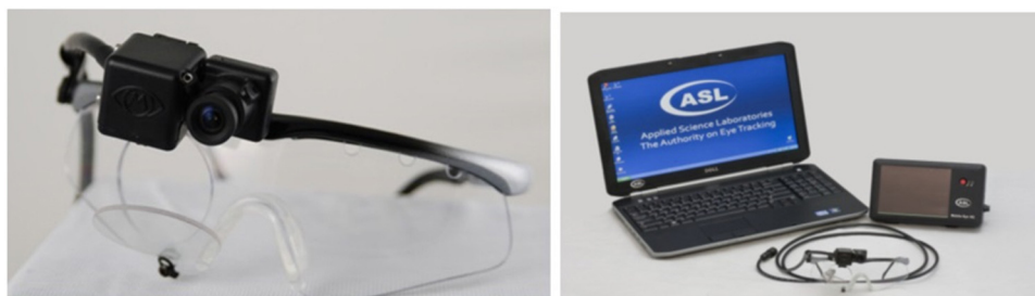
Fig. 1. ASL Mobile Eye XG Glasses on the left, complete equipment with DTU on the right.
